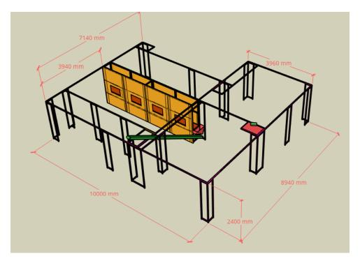
The set is a selfstanding aluminum construction in total 10m by 9m, 2,40m high.
